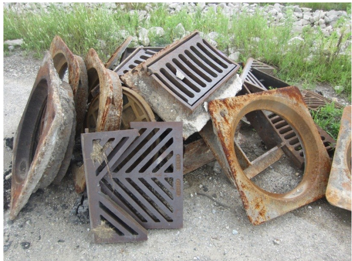
Picture 33 Broken and Removed Stormwater Grates
