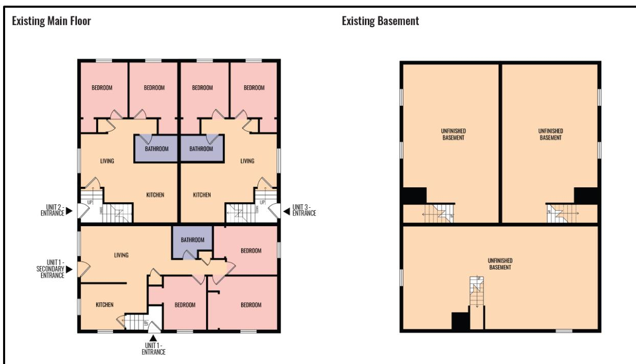
Figure 7 – Floor Plan of the existing triplexes.
