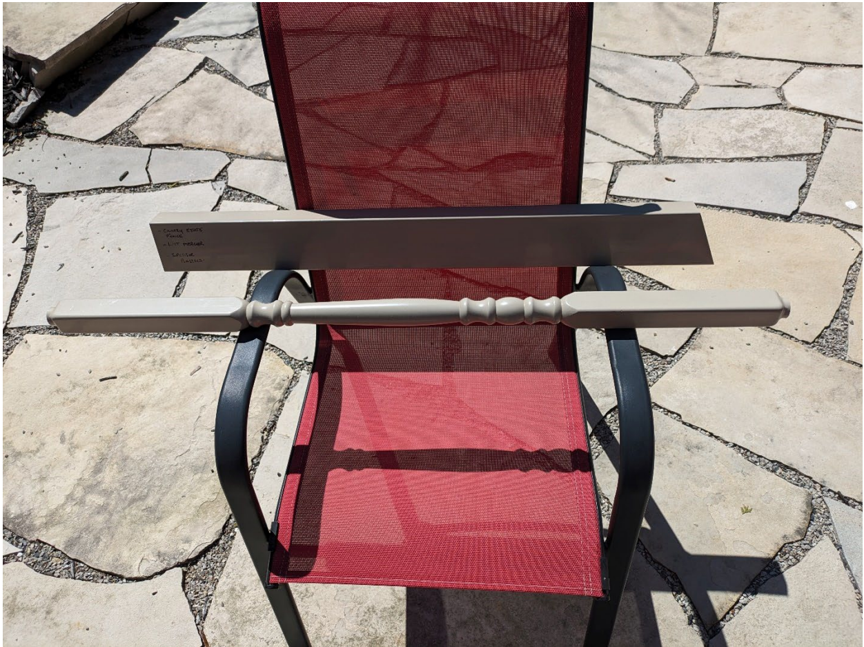
Image 5: Photograph submitted with the Heritage Alteration Permit application showing proposed vinyl (Country Estate 1.5" x 1.5" Vinyl Spindle Railing") replacement railing materials.
