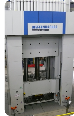
Dieffenbacher hydraulic high-speed press with a maximum press force of 25,000 kN (2,500 tons)
