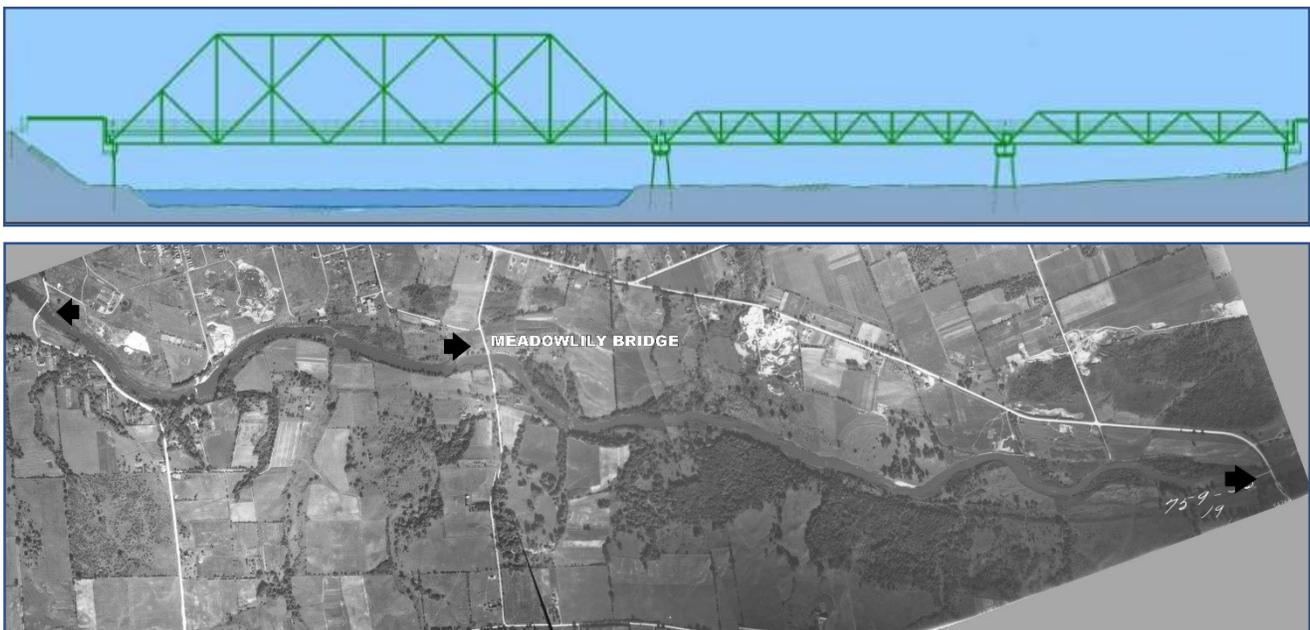
21. (top) Meadowlily Bridge elevation diagram showing the main span and two flood plane spans, With the so called through-truss design the road bed literally runs through the interior of the truss. Credit: HistoricBridges.org
