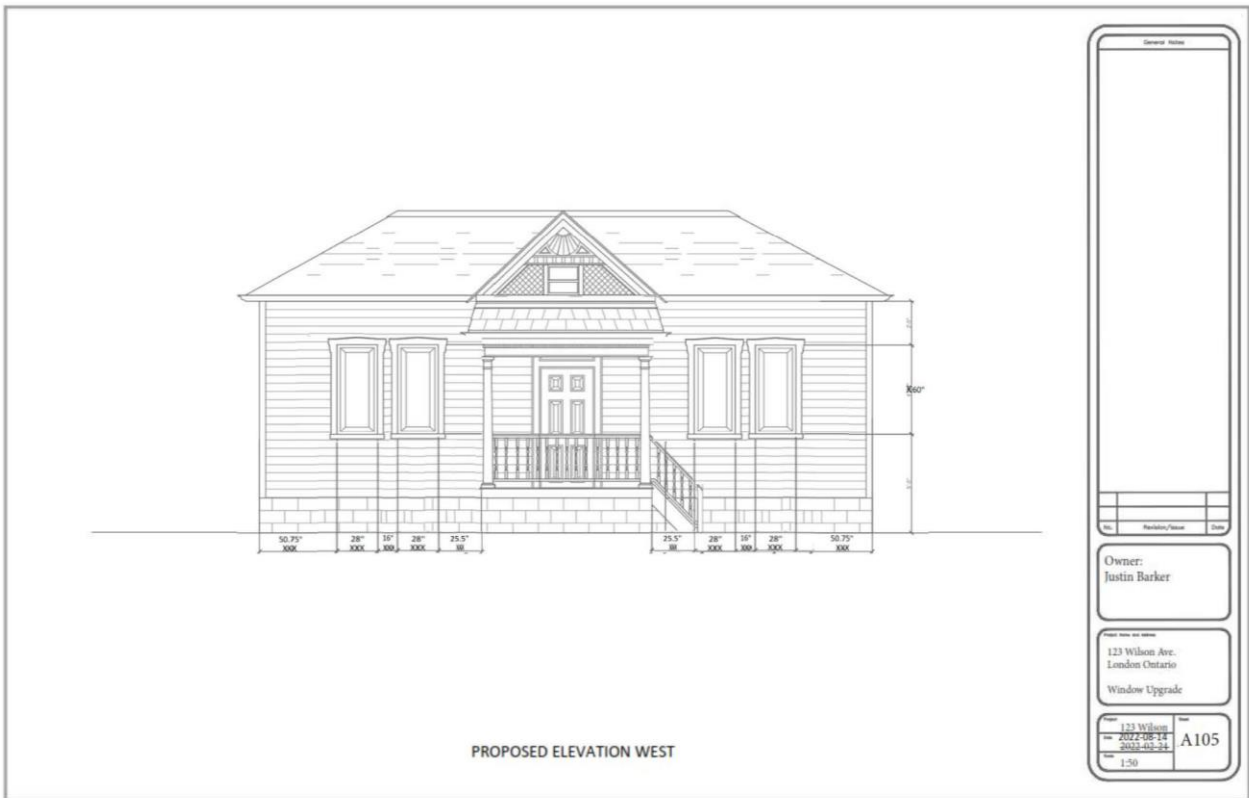
Figure 3: Proposed floor plan, submitted as part of the Heritage Alteration Permit application. Showing the proposed reinstatement of the four windows on the west façade as well as the existing window on the south façade.
