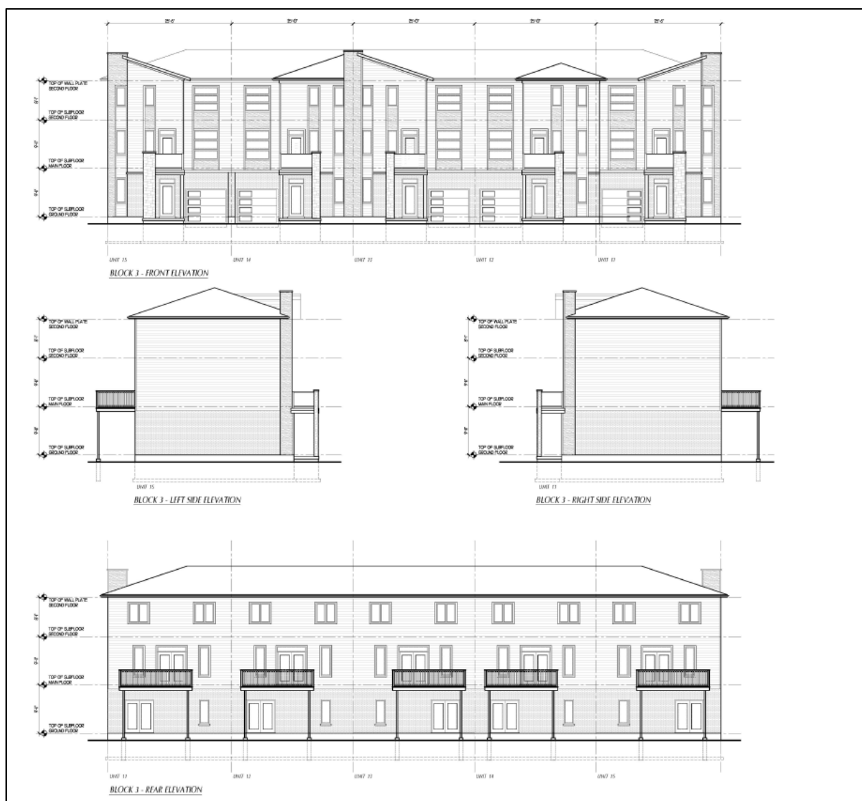
Figure 4: Concept elevations – units internal to the site with second storey decks.
