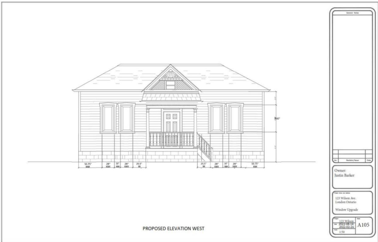
Figure 4: Proposed west elevation drawing, submitted as part of the Heritage Alteration Permit application. Showing the reinstated five-bay design with replicated window trim. Note: the proposed replacement windows must include the two-over-two fenestration pattern of the former windows (not shown on the above drawing).
