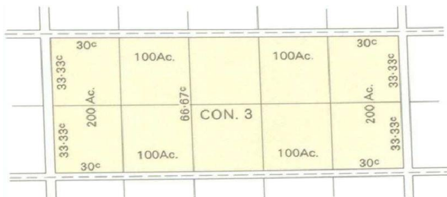
Plate 1: Double Front Survey System (Dean 1969)
