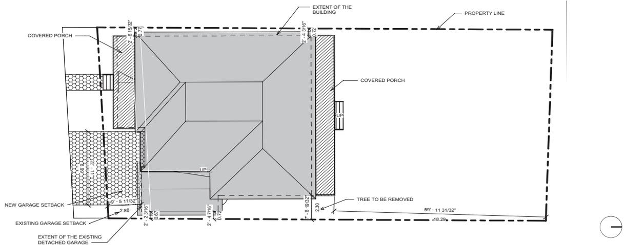
Image 22: 18 Byron Ave E. proposed site plan with parking for two vehicles to the south/front of the site. HCD plan recommends two single track driveways with turf installed between in order to minimize the impact of hard surfacing. Drawing by Third Layer Architects, 2021.
