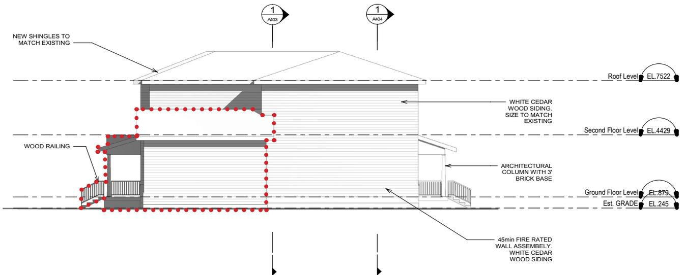
Image 21: East Elevation. Red dotted line indicates outline of existing garage and front porch (beyond) to be incorporated into proposed addition/renovation. Drawing by Third Layer Architects, 2021.
