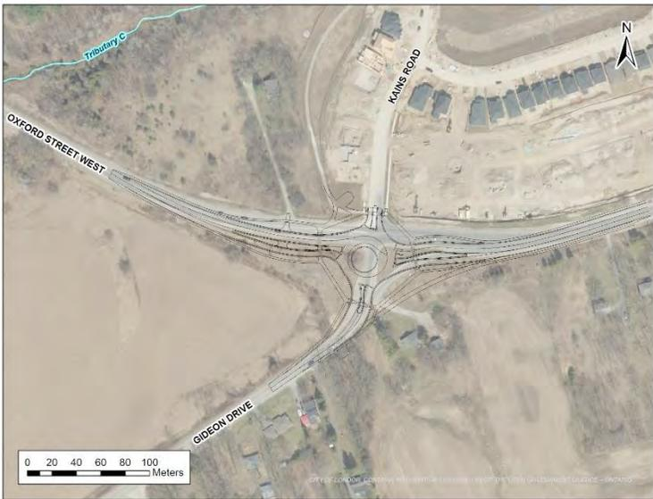
**Figure 7.4 – Alternative Solution 4 – Multi-Lane Roundabout**
