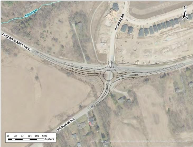
**Figure 7.3 – Alternative Solution 3 – Single-Lane Roundabout**
