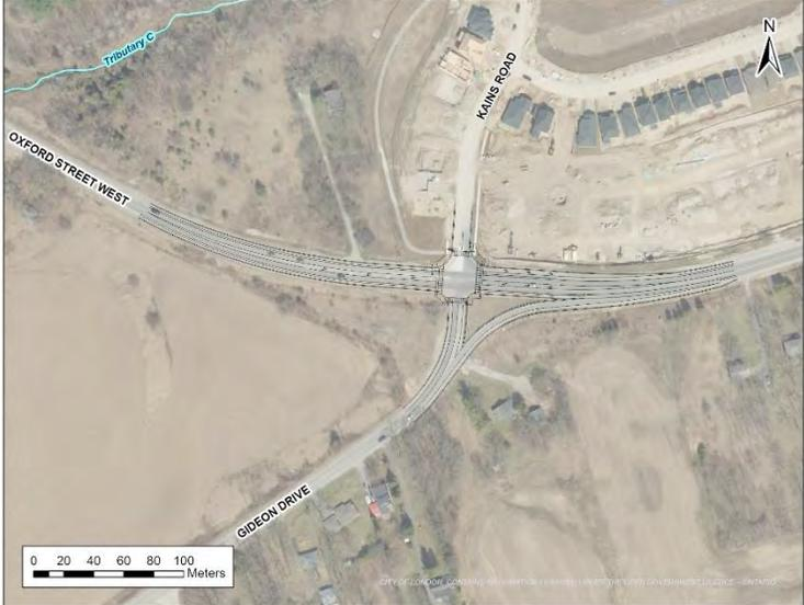
Figure 7.2 – Alternative Solution 2 – Signalized Intersection
