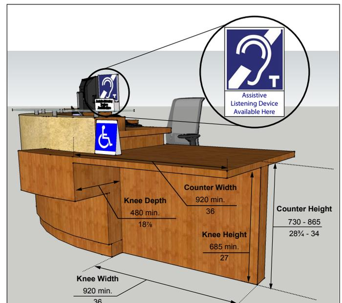
Figure 110: Dimensions of Accessible Service Counter
