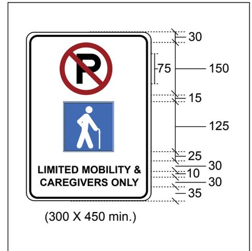
**Figure 27c:** Type C Vertical Signage - Detailed Dimensions
