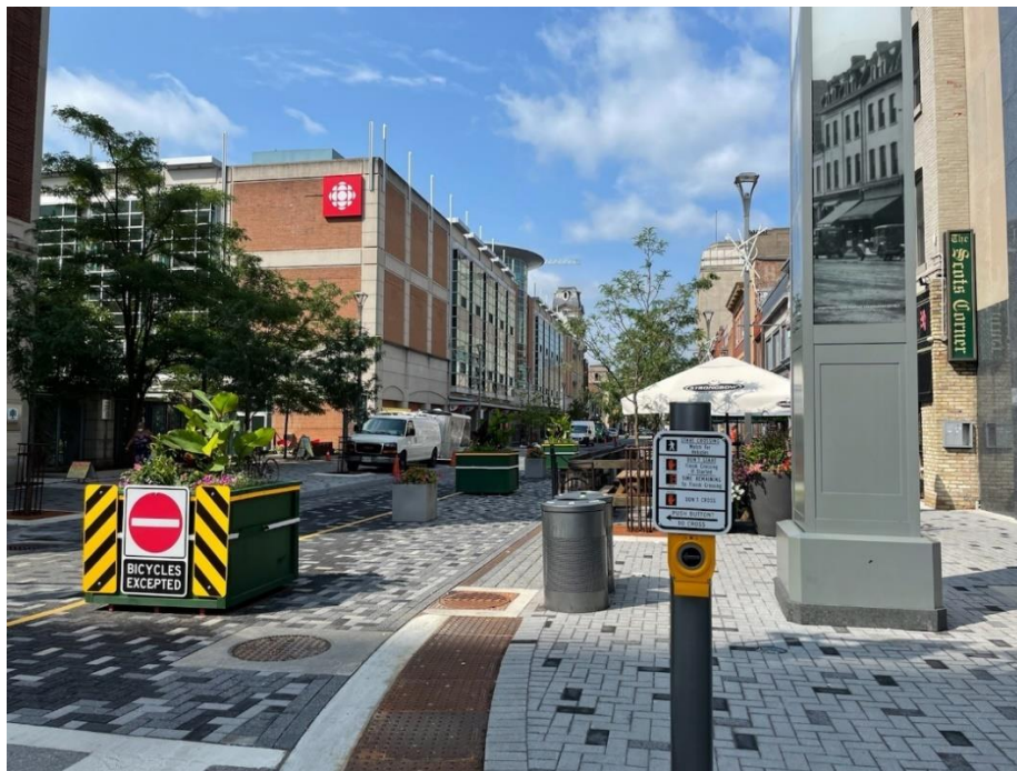
Figure 2: Planter barriers and signage installed to restrict motor vehicles from entering Dundas Place from Wellington Street.
