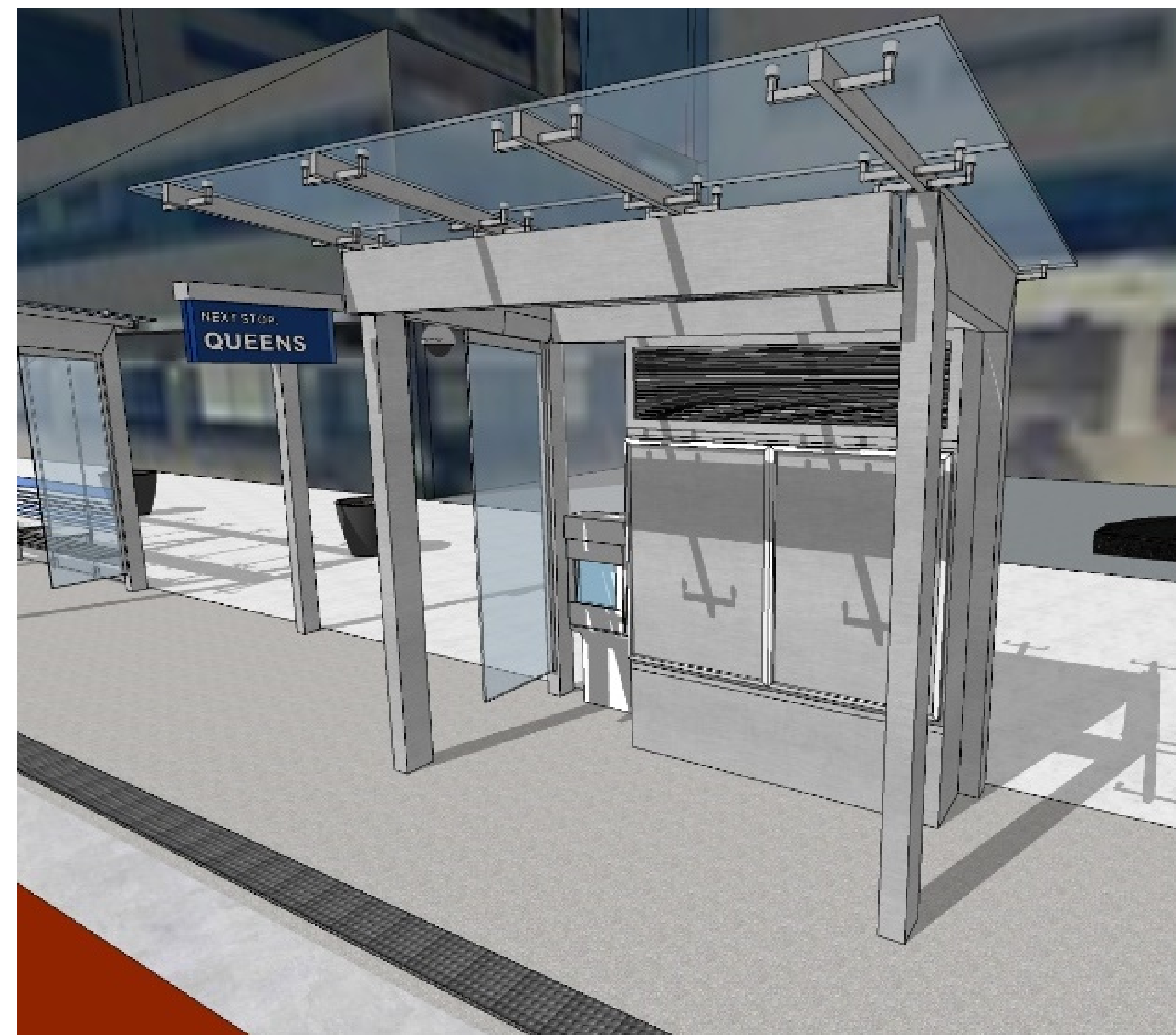
Ticket vending machines and message signs
