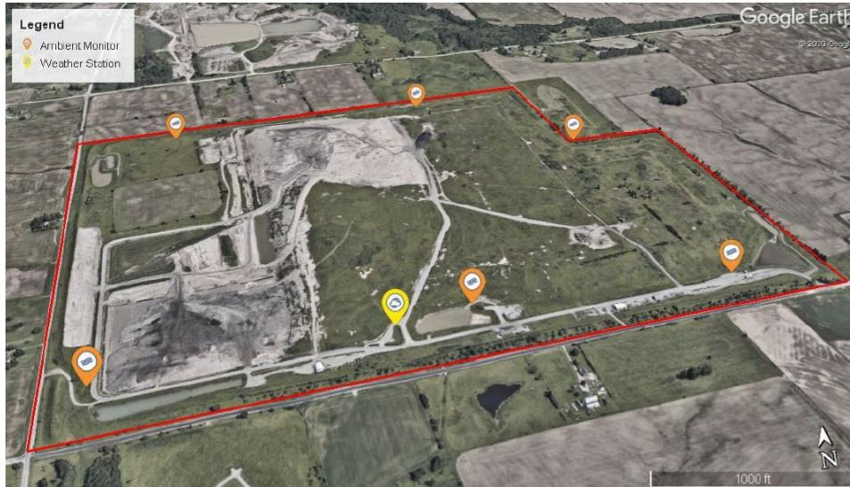
Landfill gas contains hydrogen sulphide, known for its distinctive "rotten egg" odour, as well as organic sulphur compounds known as "mercaptans" known for their "putrid" odour. The ambient monitor measures both hydrogen sulphide and methyl mercaptan and reports these as equivalent hydrogen sulphide.
