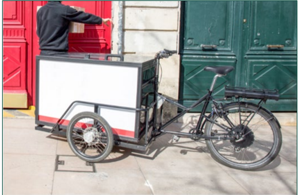
Reverse tricycle design with enclosed cargo box in the front
