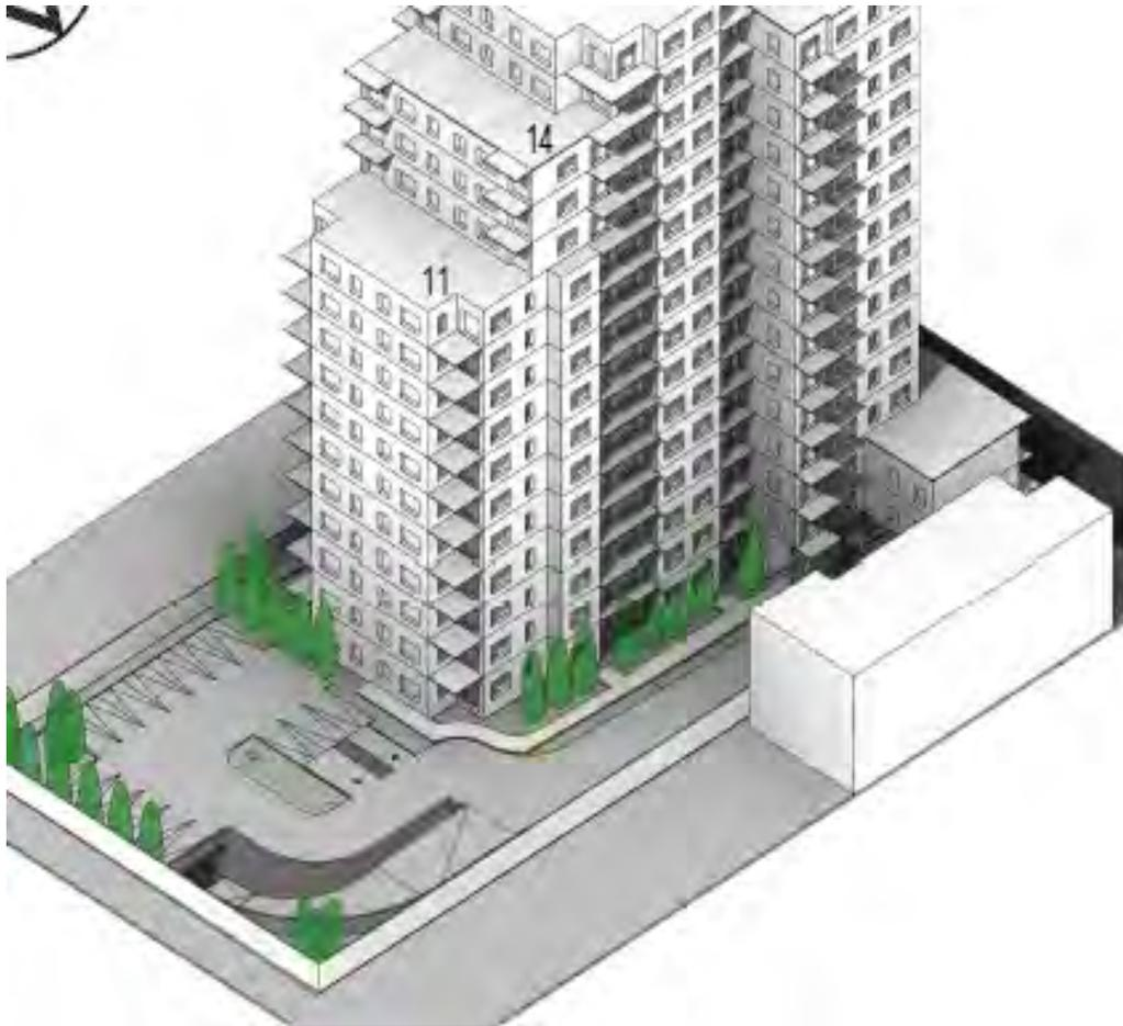
**Figure 29**– (Above) Massing model of proposed development looking westward showing stepbacks on third and 15<sup>th</sup> floor; (Below) Massing model from the rear demonstrating stepbacks on the 11<sup>th</sup>, 14<sup>th</sup> and 16<sup>th</sup> levels (Source: Zedd Architecture, 2020)
