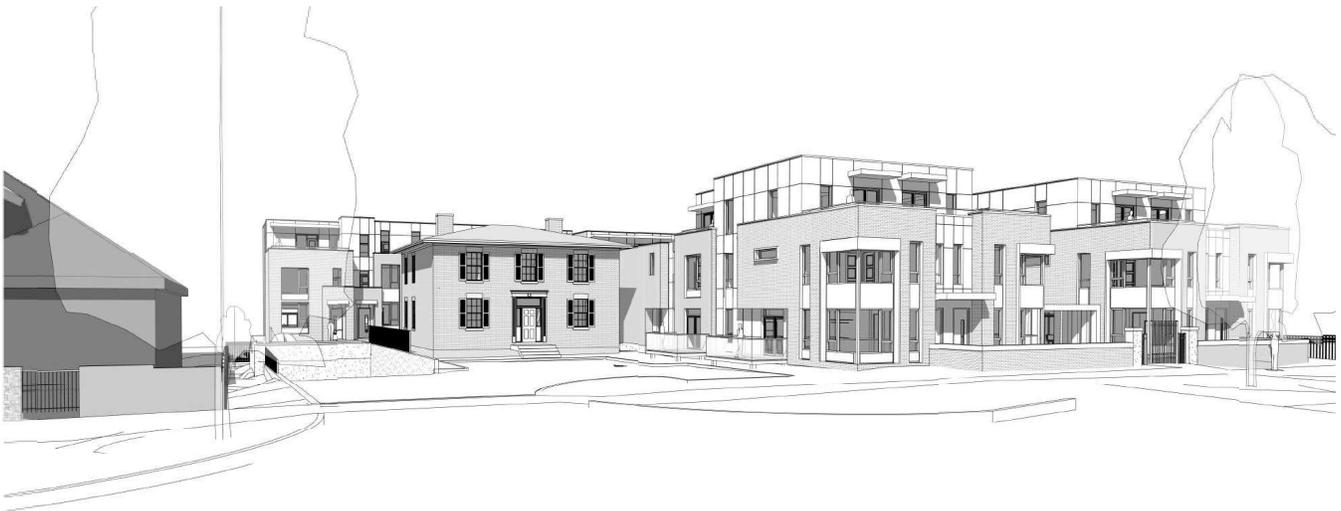
Rendering of 2096 Wonderland Road N. proposed development of townhouse condos located around the existing heritage house, in-situ. Retention of the existing designated heritage property in-situ is proposed by way of raising the structure to remove the existing foundations and construct new foundations. A proposed underground parking lot not pictured will be located adjacent to the heritage home. Drawing by ZEDD Architecture, Nov 2020.
