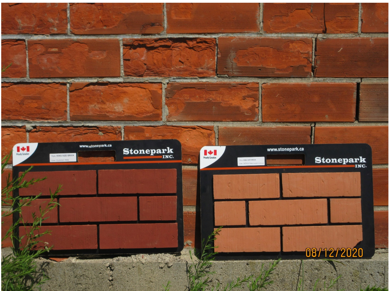
Image 3: Photograph showing two samples of a proposed veneer cladding, seeking a suitable colour match. The sample on the left has been selected as the preferred veneer cladding.
