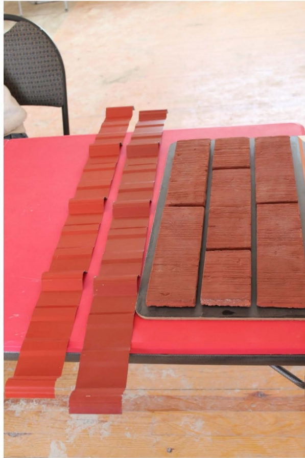
Image 4: Photograph showing the proposed veneer cladding for the new exterior walls of the barns, as well as two samples of a corrugated sheet metal roof.
