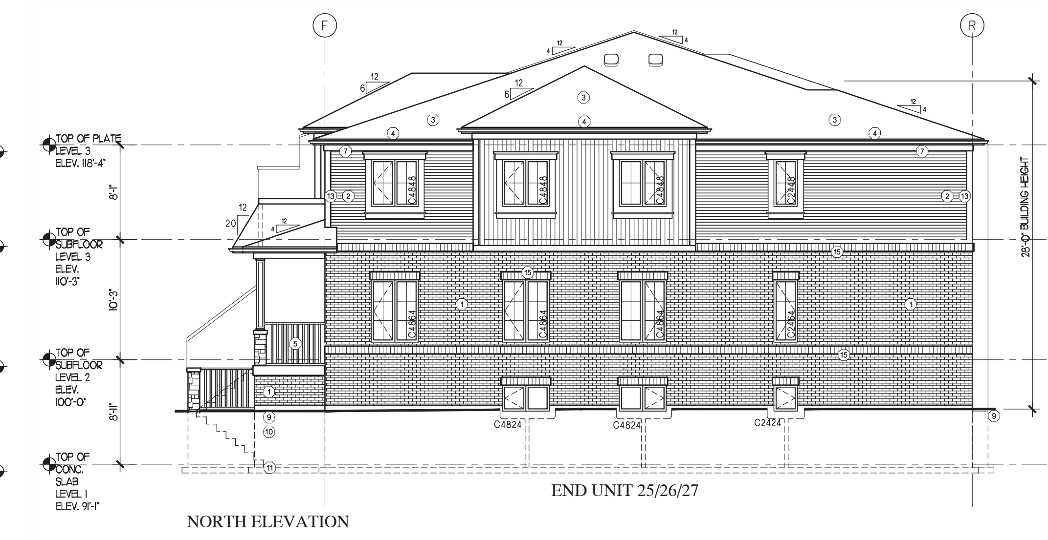
NORTH ELEVATION END UNIT 25/26/27
