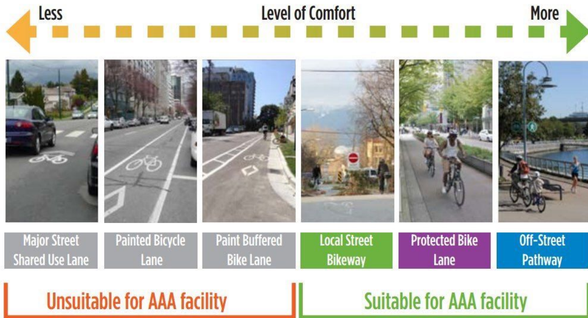
Figure 6-2: City of Vancouver guidelines for All Ages and Abilities Cycling Network Design. Off-street pathways must be brightly lit, and maintained through four seasons to be considered effective. 53
