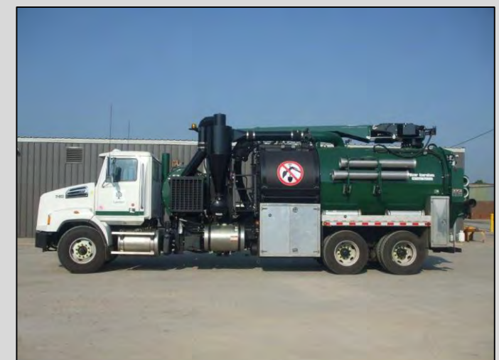
London Fleet – Sewer Cleaning Truck
