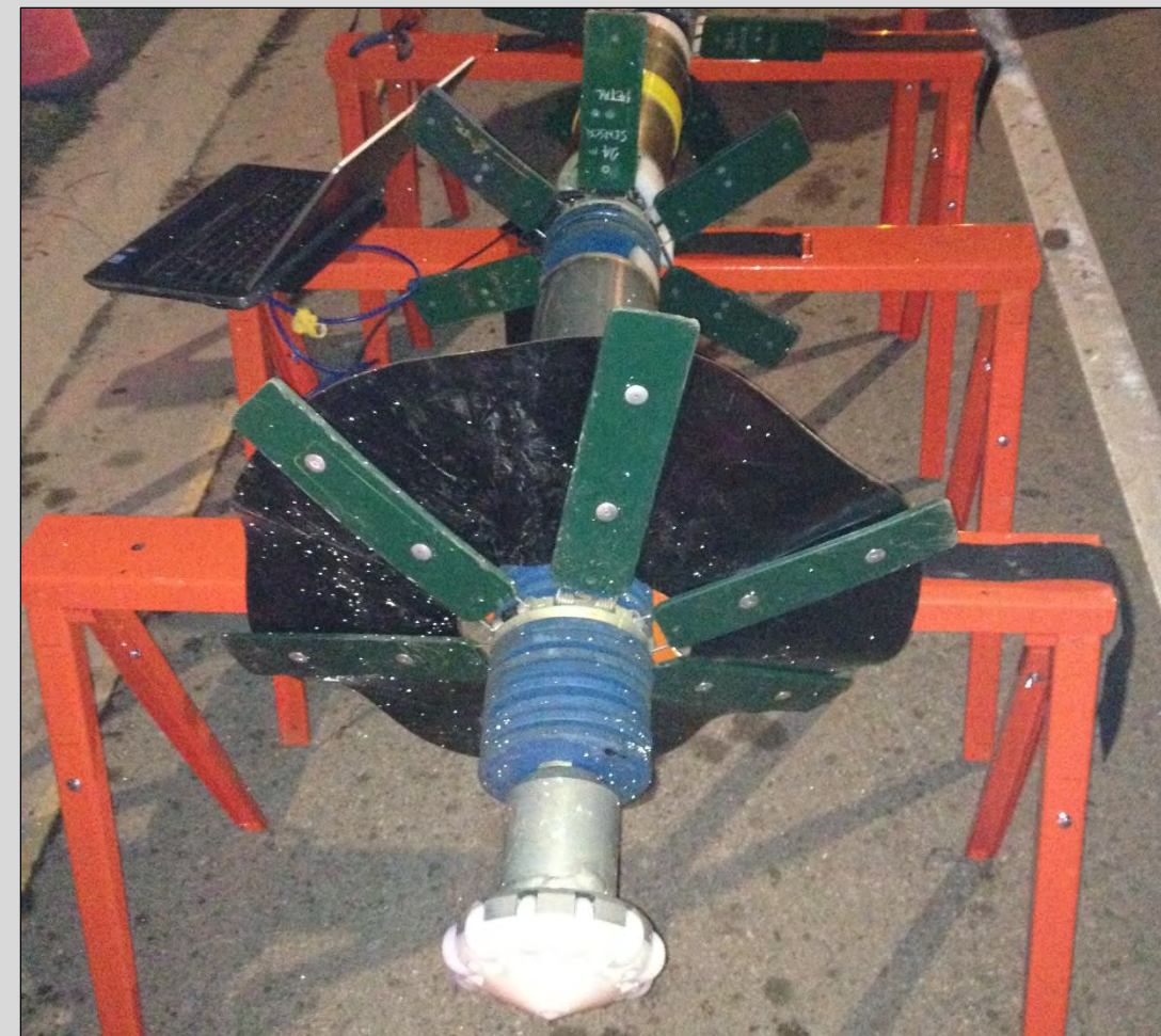
PipeDiver used to inspect live watermains
