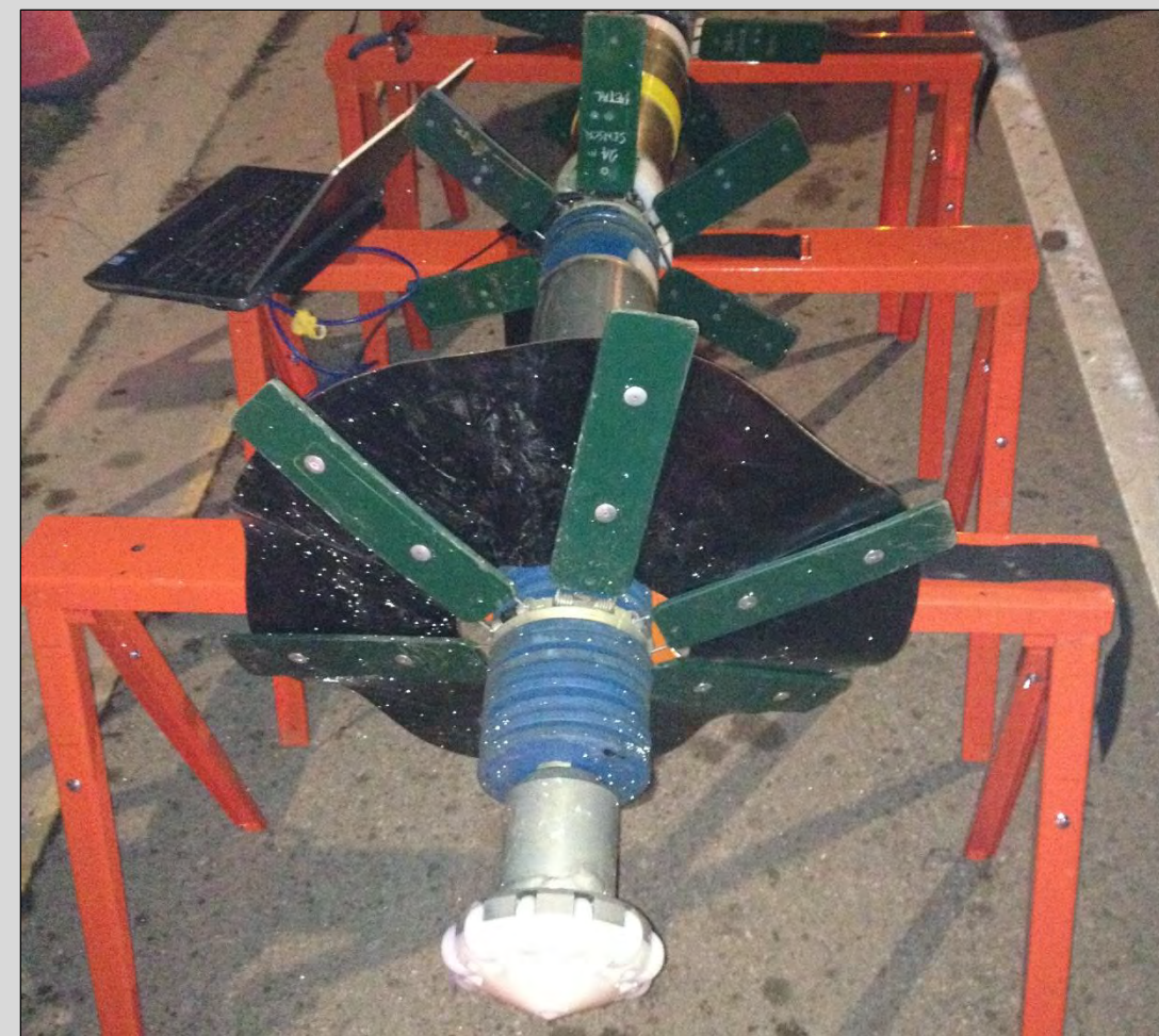
PipeDiver used to inspect live watermains
