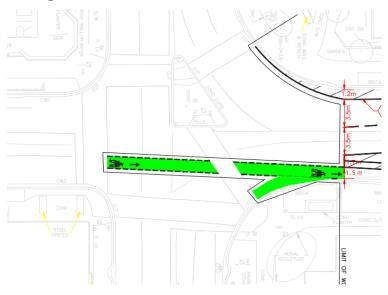
Intersection treatments will be similar to Colborne Street cycle track with green bike boxes and green cross rides along the intersection. A two-stage queue box is planned to be installed on Colborne Street for cyclists making left turns. There are several driveways throughout the King Street corridor and these mid-block conflict locations will be painted green similar to Colborne Street.
