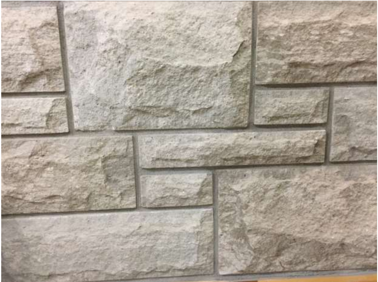
Image 11: Photograph of the proposed composite stone for the cladding of the base of the proposed detached garage (Arriscraft International, random three-unit "Laurier Building Stone" in mahogany colour). Courtesy Myk Wasylko, Wasylko Architect Inc.
