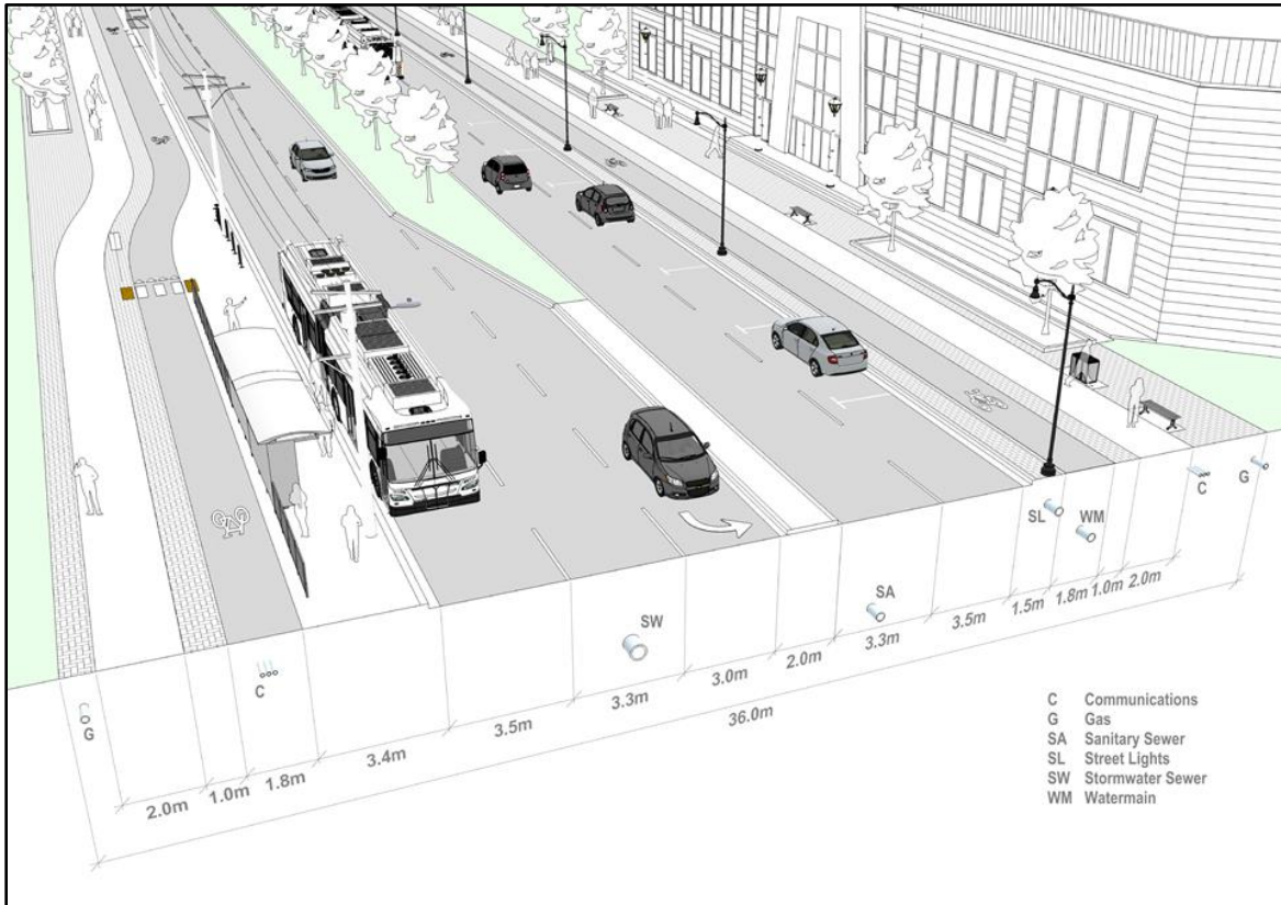
Civic Boulevard Typical Cross-Section
