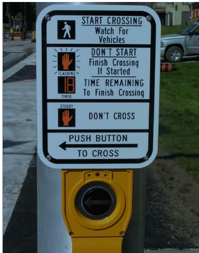
An AODA compliant push button
