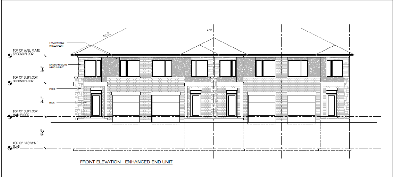
2-storey townhouse front elevation
